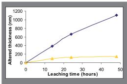
Figure 1: Evolution of glass alteration: comparison between a usual tracer (Boron) and Gold implanted.
