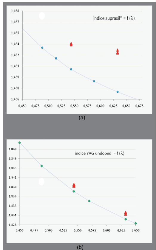
Fig-1: accuracy of the M-Lines spectroscopy
