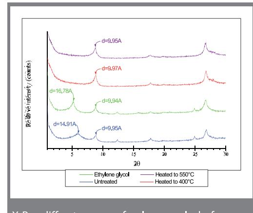
X-Ray diffractograms of a clay sample: before treatments, after an ethylene glycol treatment, after a heating at 400°C and another at 550°C
