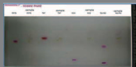
Figure 2 : HPTLC plate of samples extracted with acetonitrile and washed with hexane Developing solvent : trichloroethylene/acetone Hexane phase
