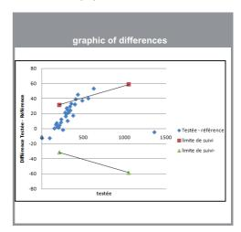
The automat overcomes the errors from the manual method currently used. This graph attests that the manual method under estimated the quantification of citric acid in urine. Lots of parameters like the homogeneity of sample, the temperature of the reaction, the accuracy of the swab are controlled with the automat. Moreover this automated method doesn't require preparation of samples and a kit for citric acid in urine is used.
